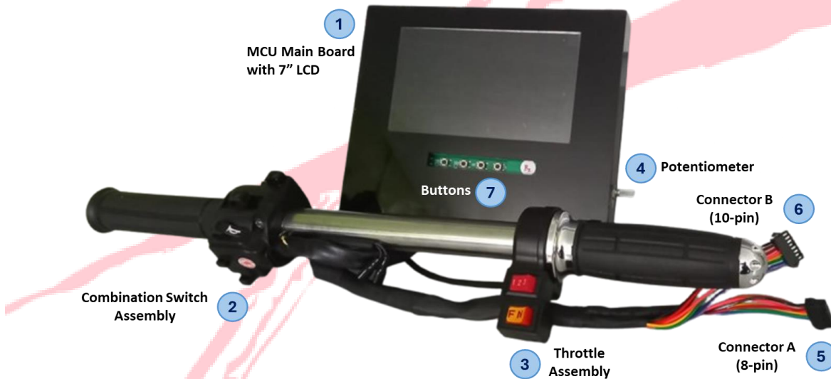
Figure 2 Parry's Digital BLE Cluster Reference Solution
